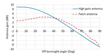
Figure 5: PROBA-3 receiver antenna patterns. Nadir-pointing patch antenna pattern and zenith-pointing high-gain antenna pattern.
