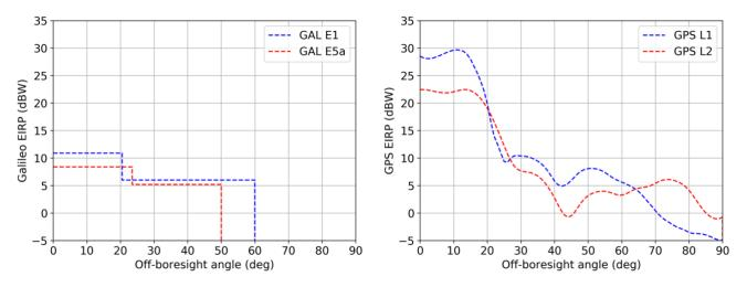
Figure 4: ESA/ESOC non-official Galileo E1 and E5a EIRP models on the right and GPS L1 (ACE) and L2 (Lockheed Martin) EIRP values on the left-hand side as a function of the off-boresight angle.
