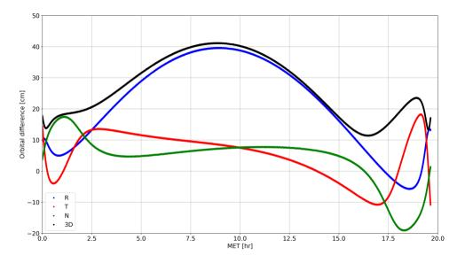
Figure 8: POD absolute orbital difference RMS for the single frequency GRAPHIC linear combination scenarios for a CN0 threshold of 20 dB-Hz.
