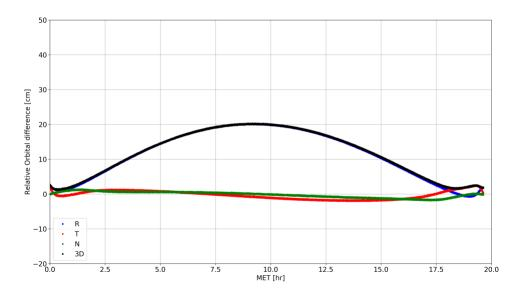
Figure 9: POD relative orbital difference RMS for the single frequency GRAPHIC linear combination scenarios for a CN0 threshold of 20 dB-Hz.
