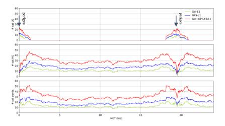
Figure 6: GNSS signal availability for a CN0 receiver threshold of 20dB-Hz for the Galileo E1 and GPS L1 frequencies.
