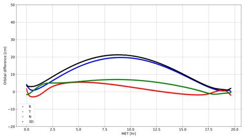
Figure 10: POD absolute orbital difference RMS for the dual frequency ionospheric-free linear combination scenarios for a CN0 threshold of 20 dB-Hz.
