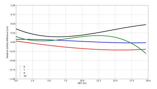
Figure 11: POD relative orbital difference RMS for the dual frequency ionospheric-free linear combination scenarios for a CN0 threshold of 20 dB-Hz.
