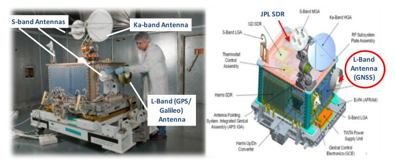
Installed on the International Space Station (ISS) in July 2012 Fully reprogrammable Software Defined Radio capability at L-band
