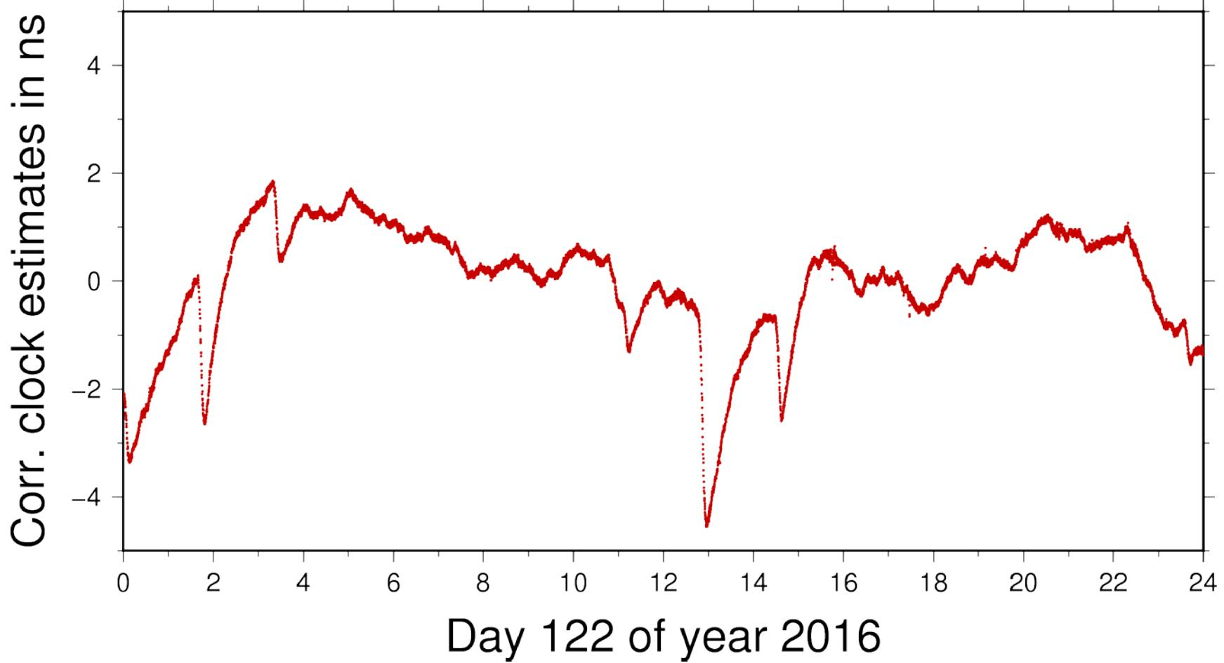
From the corrected (jumps and relativistic effects) receiver clock estimates a quadratic model has been subtracted.
