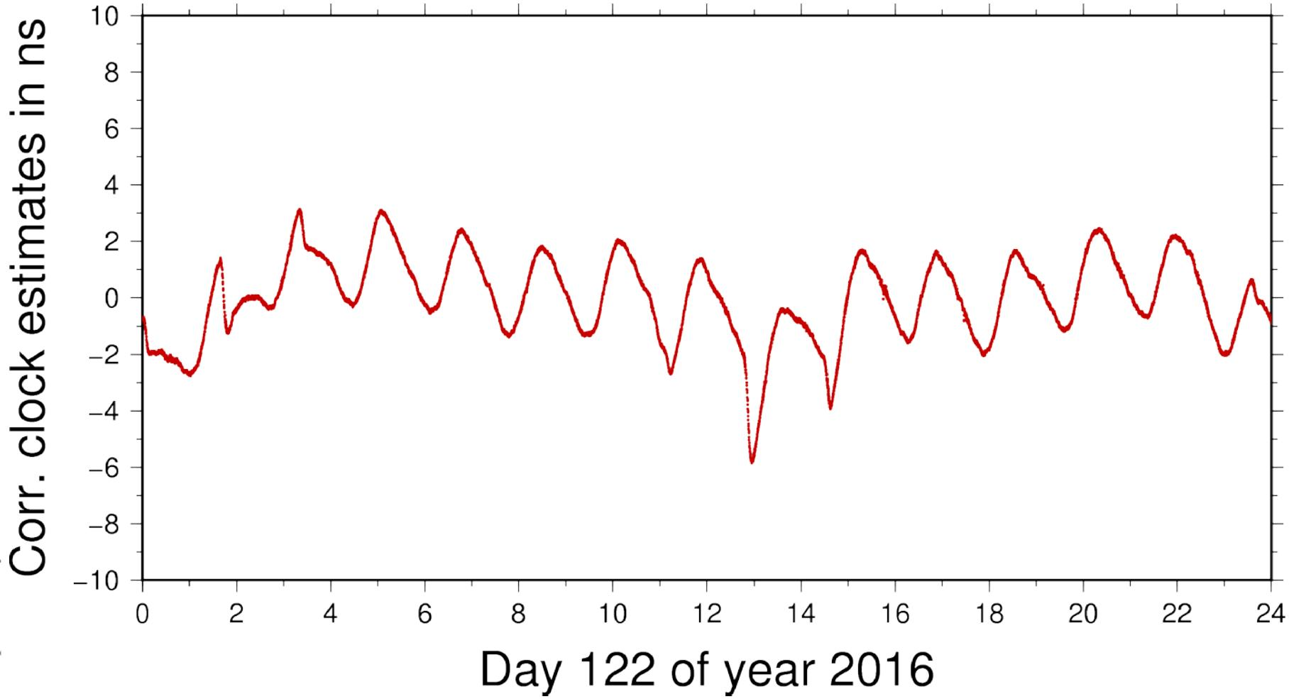
From the corrected (jumps) receiver clock estimates a quadratic model has been subtracted.
