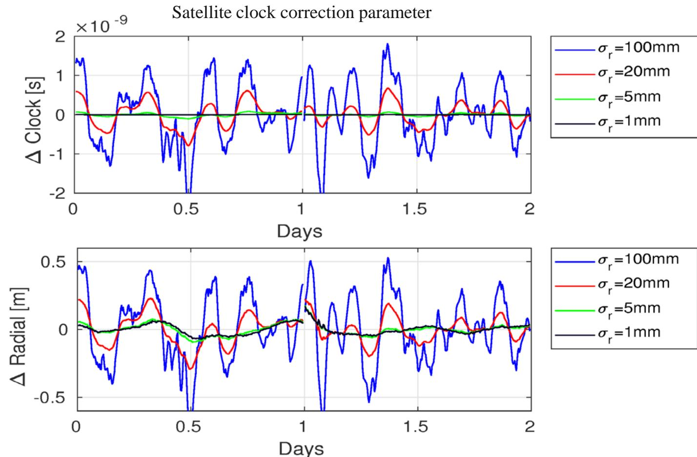
Difference of the radial component between the kinematic estimated orbits and the dynamic reference orbit.
