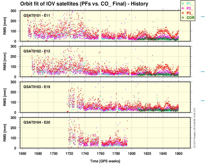
Difference between PF and CO\_ Galileo orbits are in the range of 5 to 15 cm (with outliers in case of data problems)
