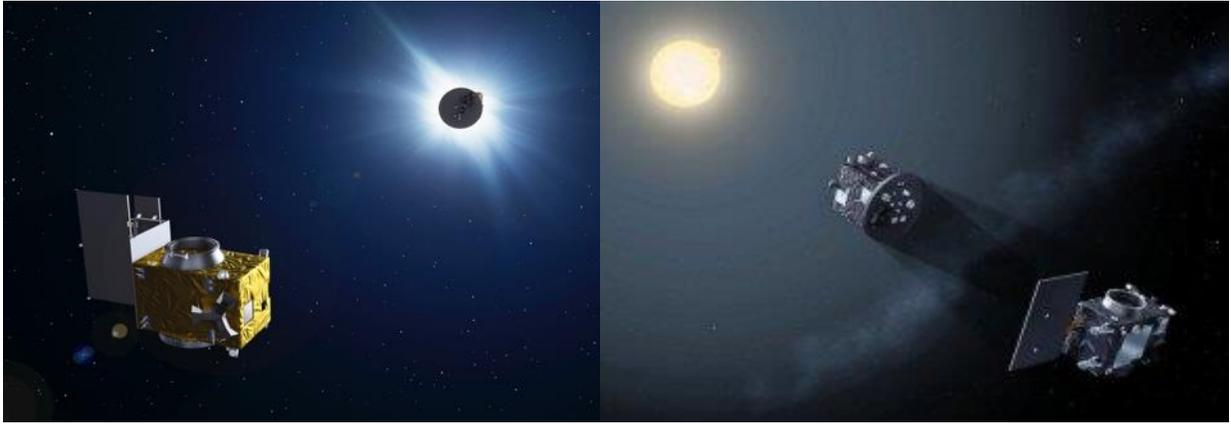
**Figure 1: Principle of PROBA-3 solar coronagraph science experiment**
